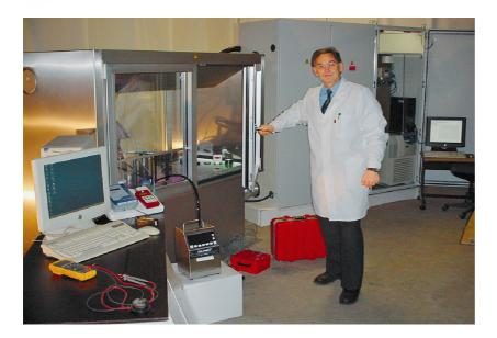
The sensitive heart of any project is the ultra micro balance (accuracy about  $1 \mu g$ , left inside the chamber).
